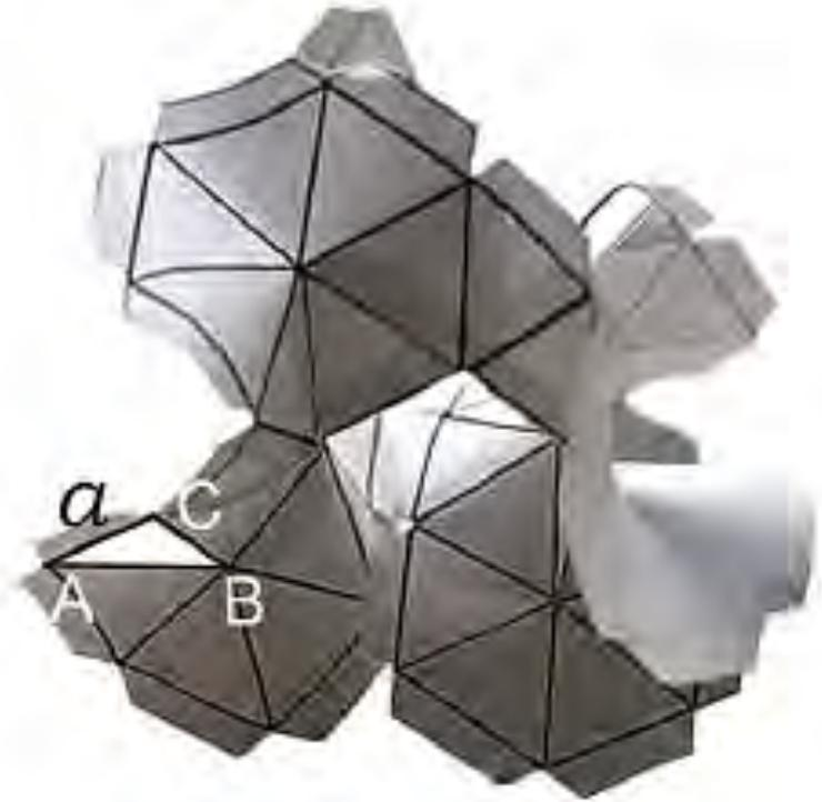
When we open the slit, the material relaxes into the 3D structure
